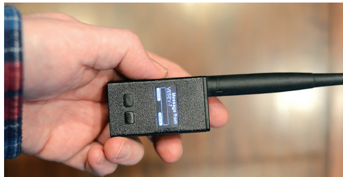
Figure 5 — The PicoAPRS has a standard SMA female antenna jack and can be used with any 2-meter antenna. Here it's shown with the flexible antenna from the author's dual-band handheld transceiver.
